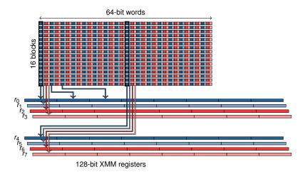
Packing for the 16-parallel bitslice implementation of LED and PRESENT.
