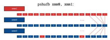
vperm for short, was introduced by TWINE designers in SAC 2012, takes advantage of SIMD (single instruction multiple data), especially "pshufb" instruction, introduced with SSSE3 extension with Intel Core microarchitecture.
