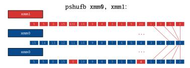
When xmm0 stores s[0], s[1],..., and sbox inputs are stored in xmm1 byte-wise, then this instruction functions as substitution byte-wise, in parallel. Perfectly fits 4-bit sboxes, with possibility extending to larger outputs.
